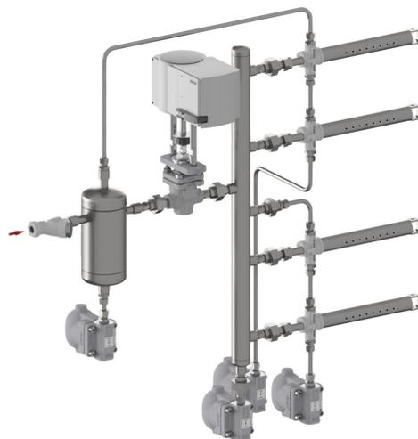
Recommended when the sum of insertion lengths (dimension "C") totals more than 7 meters.
