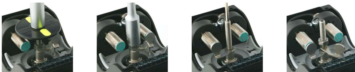
Fig. 4 – Adjusting cams in cylindrical limit switches
