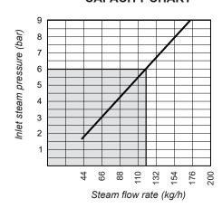
Remark: Selection under shadow area is recommended. Capacities shown are valid for vessels which are vented to atmosphere.
