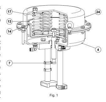
The amount of pressure required to stroke the actuator between its rated travel positions is established by the spring range, which depends upon the spring quantity and force and the diaphragm effective area.
