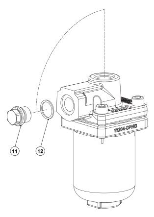
Fig. 2: Outlet flow direction change.
