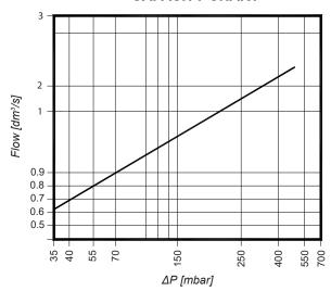
$\Delta P$  required to open vacuum breaker: 6,13 mbar.
