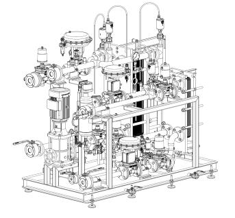
Compact and modular design, easy to transport and install skid mounted systems either for heating or cooling service.
