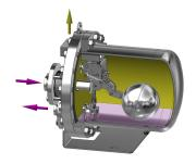
1. In the first instance, the steam intake valve is closed, while the vent valve is open. As condensate flows into the body through the inlet check valve, the PPT14 can operate in a closed loop application, in one of two ways (as a steam trap or pressure operated pump).
