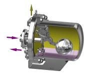
6. As the motive steam valve closes and the vent valve opens, equalizing the body pressure with the upstream pressure, the condensate is allowed to flow once again into the PPT14. The cycle then repeats itself and, with enough differential pressure, the PPT14 resumes as a steam trap or, otherwise, as a pump.
