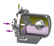
3. As soon as, e.g., the equipment control valve starts to modulate, the steam pressure will decrease. The lower differential pressure decreases the PPT14's ability to discharge as a steam trap causing the condensate level to rise inside the body. Vacuum may even occur at this stage.
