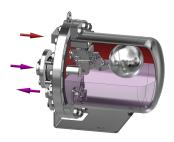
4. If this situation would persist, the condensate would eventually flood the equipment, causing problems. However, by using a PPT14, as the float reaches its highest position, the snap action mechanism actuates, closing the vent valve and opening the steam intake valve. Steam will then replace the necessary positive pressure to pump out the condensate. At this point the PPT14 works as a pressure operated pump.
