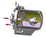
2. If the inlet pressure is greater than the back pressure, the PPT14 works as a steam trap, continuously discharging condensate by differential pressure. At this point the steam intake valve remains closed and the vent valve open.
