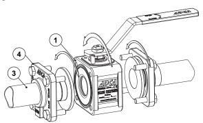
Fig. 2 - Tube weld ends with loose flanges.
