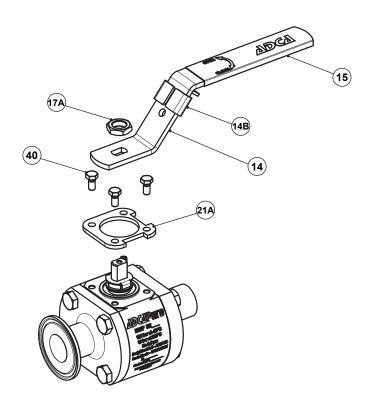
Fig. 7 - Valve with lockable lever.
