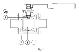
For manual valves, operation is performed by turning the handle by <sup>1</sup>/<sub>4</sub> turn to "fully close" or "fully open" the valve. The valve is "fully open" or "fully closed" when the handle is parallel or perpendicular to the pipeline respectively.
