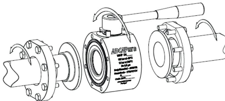
Loose body flanges make it possible to install the valve without aligning of the welded end connections. After installation the valve can rotate on 360° for the desired orientation.
