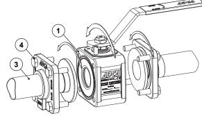
Fig. 2: Tube weld ends with loose flanges.
