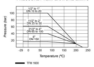
Remark: Maximum operating conditions may be limited by the valve end connections due to normative restrictions.
