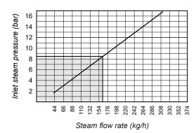
Remark: Selection under shadowed area is recommended for the quietest operation.
