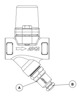
Fig. 2 - BM series steam trap installed with BDV blowdown valve.
