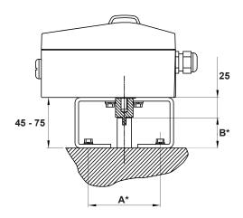
\* Dimensions A and B are dependent on the rotary actuator.
