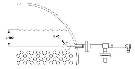
Remark: Provide a spacing of at least 40 mm between the probe central electrode pole and any metallic parts such as the boiler wall, tubes and other metallic fittings. The probe must be installed in such a way that it is always in contact with water and wetted parts fully immersed, without air gaps. As far from the feedwater inlet as possible and away from the steam bubbles, at least 100 mm below the boiler low water level.
