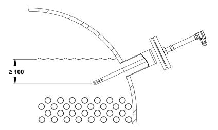
Remark: Installation at a 45° angle, only possible when probe is fitted with a threaded outer shroud.
