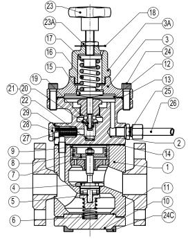
Regulators occasionally give trouble (particularly on new installations) due to dirt and other foreign matter fouling the internals. In this event, the trouble can often be quickly eliminated by applying the following first aid treatment:
