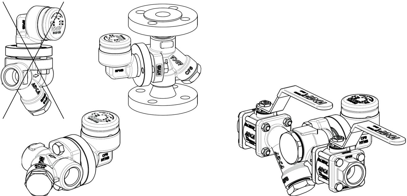
*UDT46 steam trap connected to a UCX universal pipeline connector*
