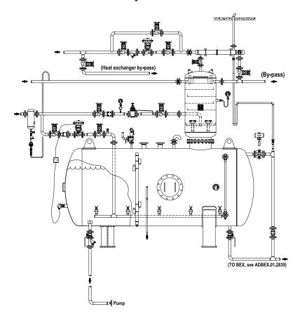
Thermal deaerators, including ADCATherm STS series complete stainless steel heat exchanger. Make-up water crossing the heat exchanger will condense the flash steam, preventing energy waste and increasing performance of the whole system.
