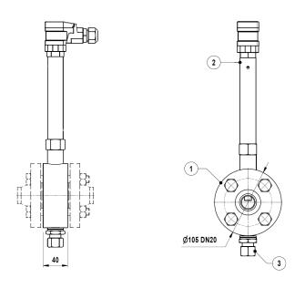
Remarks: Can be fitted into a "T" connection or into our standard chamber, providing that the probe is always in contact with the water. Any metallic parts near the probe must be at a minimum distance of 20 mm from the central end pole.
